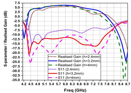
**Fig. 9:** Simulated reflection coefficients and realised gain for different sizes of substrate height.
