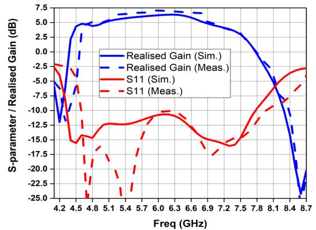
**Fig. 18:** Simulated and measured reflection coefficients and realised gain of the proposed antenna.
