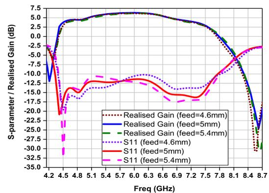
**Fig. 10:** Simulated reflection coefficients and realised gain for different positions of feeding probe.
