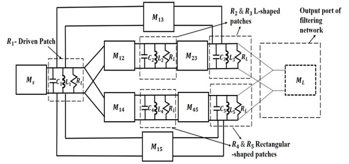
**Fig. 5:** Circuit model of the proposed antenna where the output port (dotted lines and  $M_L$ ) is added when the filtering network response is calculated ( $S_{12}$ ).
