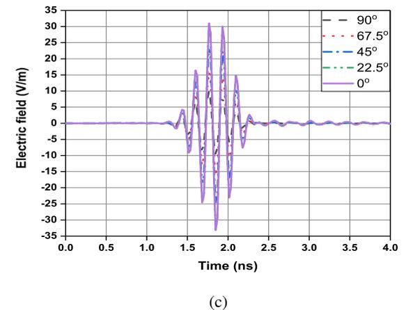
**Fig. 21:** Simulations responses of the proposed antenna (a) amplitude (dB) in different propagation directions (b) phase (degrees) in different propagation directions and (c) radiation pulses (ns) in different propagation directions
