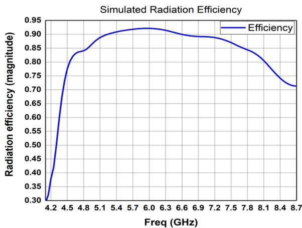
**Fig. 8:** Simulated Response of the radiation efficiency of a proposed patch antenna antenna.
