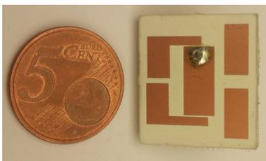
**Fig. 17:** Photograph of the fabricated proposed antenna.
