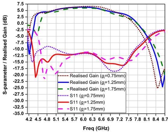
**Fig. 11:** Simulated reflection coefficients and realised gain for different gap separation of L-shaped parasitic elements and driven patch ( $g_i$ ).
