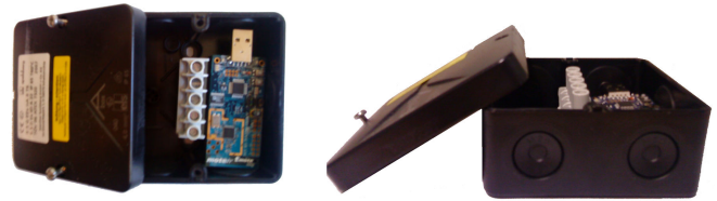
Fig. 2. A Sentilla Tmote Sky node inside an ATEX-compliant enclosure.
