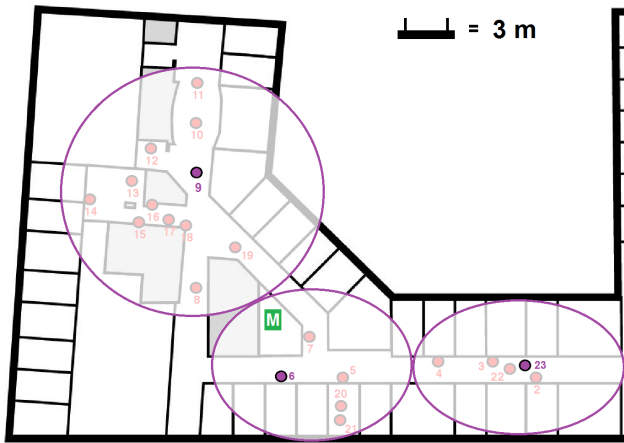
Figure 1: Testbed augmented with JamLab. Nodes 6, 9, and 23 are selected as HandyMotes, and take care of interference (re)generation in their cell.
