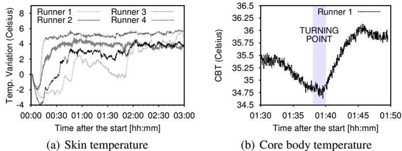
**Fig. 3.** Evolution of the skin temperature w.r.t. the start of the race (a) and impact of the wind blowing against the runners on the CBT measurements in proximity of the turning point (b).
