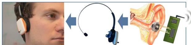
**Fig. 1.** Wireless body sensor measuring CBT at the tympanic membrane.
