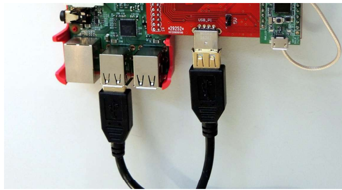
Figure 2: D-Cube, the open-source profiling tool used to benchmark the protocols. Further info can be found in [1].
