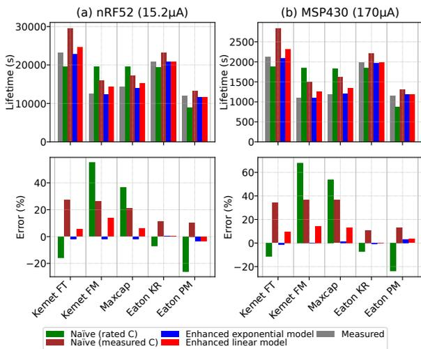
**Figure 7: Comparison of lifetime estimation approaches for two sensor nodes based on nRF52 (a) and MSP430 (b) powered by five different supercapacitors.** The enhanced linear model leads to an overestimation of the lifetime for supercapacitors with large transient leakage, but is an adequate fit for the Eaton KR and Eaton PM supercapacitor.
