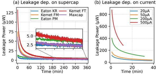
**Figure 2: Leakage profile over time for different supercapacitors at  $I_C = 0$  (a) and for a single capacitor (Kemet FT) at different load currents (b).** The leakage power is not only highly dependent on the supercapacitor model, but increases with larger discharge currents.
