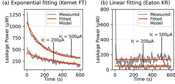
**Figure 3: Leakage profiles for the Kemet FT (a) and Eaton KR (b) supercapacitors at  $I_C = 200 \mu$  and  $I_C = 500 \mu A$ . The measured leakage can be modelled using exponential (a) or linear (b) curve fitting.**
