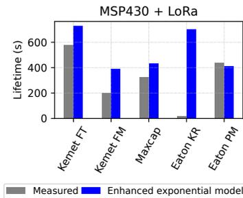
**Figure 8: Comparison of the measured and estimated lifetime for an MSP430-based LoRa node.** Due to the ESR and its effect at large load currents, the accuracy of the lifetime estimation is severely degraded.
