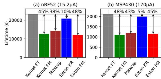
**Figure 1: Measured lifetime of an nRF52 (a) and MSP430 (b) sensor node powered by five different supercapacitors.** The two sensor nodes have an average current consumption of 15.2  $\mu$ A and 170  $\mu$ A, respectively.
