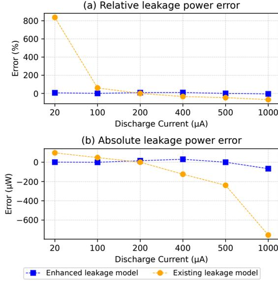
**Figure 5: Relative (a) and absolute (b) error of the enhanced exponential and existing leakage model for the Kemet FT supercapacitor.** The enhanced exponential model matches the observed leakage regardless of the used discharge current.
