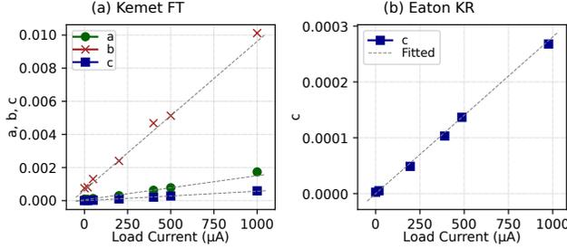
**Figure 4: Linear interpolation of curve-fitted parameters (a, b, and c) to derive a single leakage model depending on the discharge current. The linearity of the parameters allows to derive the model using only two distinct measurement points.**
