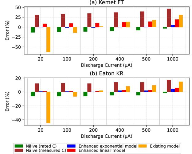
**Figure 6: Comparison of different lifetime estimation approaches for the Kemet FT (a) and Eaton KR (b) supercapacitor depending on different constant discharge currents.** The naïve approach over- or underestimates the lifetime consistently, while the error of the lifetime estimation based on the enhanced exponential model stays below 6.9% in all experiments.
