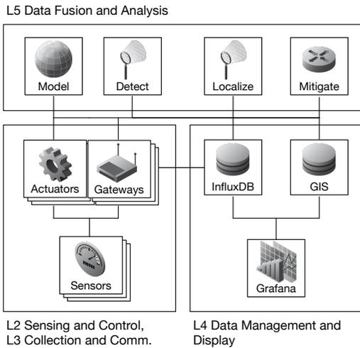
**Figure 1: Adige’s smart water network architecture classified according to the SWAN layers [18]. Layer 1 (L1) correspond to the water distribution system.**
