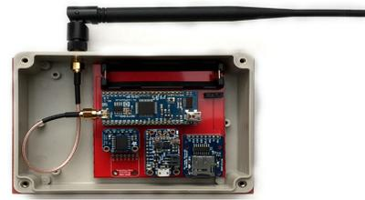
**Figure 2: An Adige Sensor is equipped with a Moteino MEGA, a real-time clock, a generic sensor interface, a power management circuit, and an SD card interface.**
