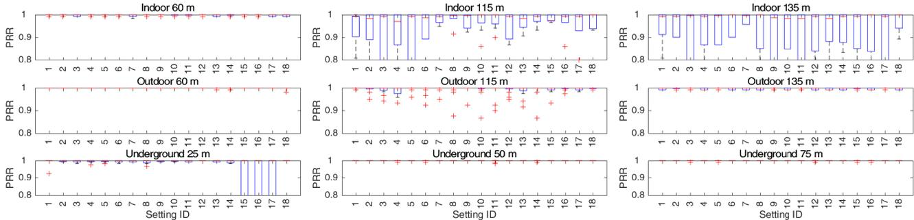
**Figure 4: Packet Reception Rate (PRR) of LoRa for different distances, scenarios and settings.**
