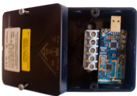
Fig. 5. ATEX case with a sensor node.
