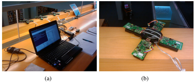
Fig. 2. The experimental setup used to collect energy level traces on IEEE-802.15.4 channels deployed at the Library of the Faculty of Engineering at the University of Porto (a) and detail of TelosB motes arranged in a USB hub (b).
