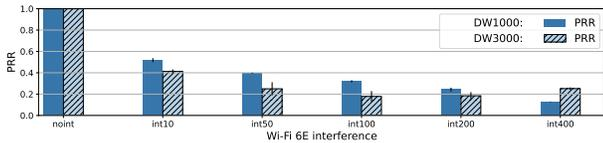
Fig. 8: Impact of different interference patterns in OFFICE.
