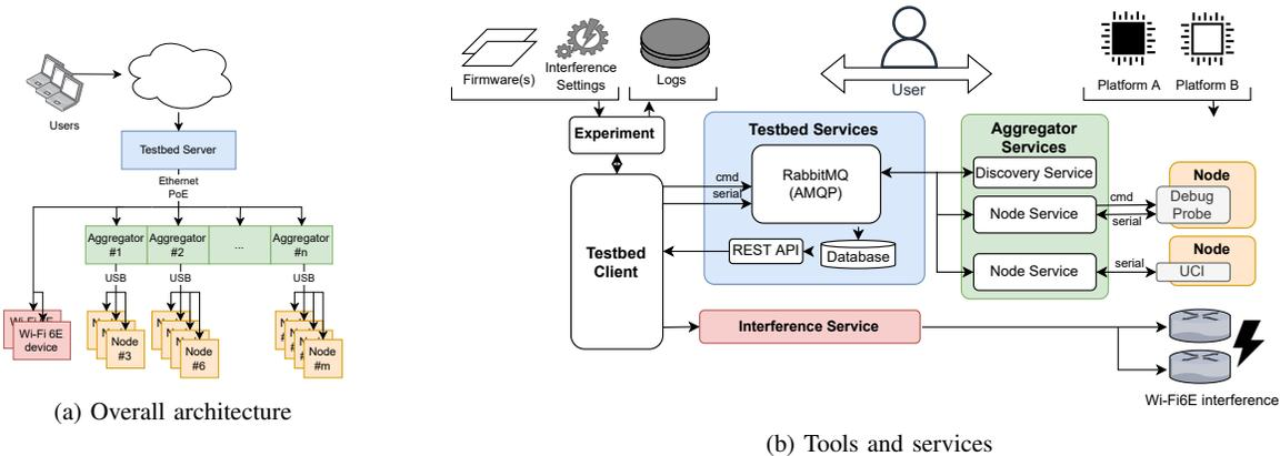
Fig. 1: Structural and functional overview of our experimental infrastructure. The architecture based on the use of aggregators allows the system to scale (a). Several tools and services provide users with an unified and hardware-agnostic way to run experiments (b).
