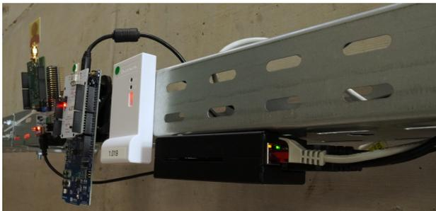
Fig. 2: Three different UWB platforms attached to an aggregator.
