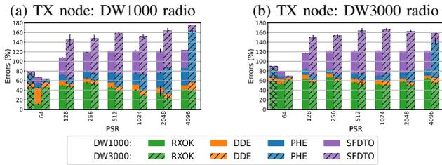
Fig. 6: PRR and reception errors for different PSR settings. The additional bar for PSR 64 refers to the DW1000’s optimized configuration.
