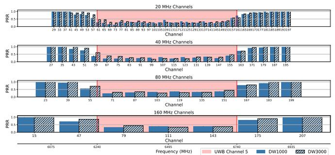
Fig. 7: UWB PRR under interference of different Wi-Fi 6E channels. Red lines mark the borders of UWB channel 5.
