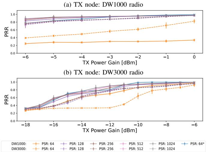
Fig. 5: Average PRR for DW1000 and DW3000 receivers as a function of the transmission power at different PSR settings. PSR 64\* refers to the optimized receiver configuration of the DW1000.
