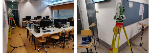
Figure 2: Example of WLOS condition (left) and NLOS condition (right) in our measurement campaign.
