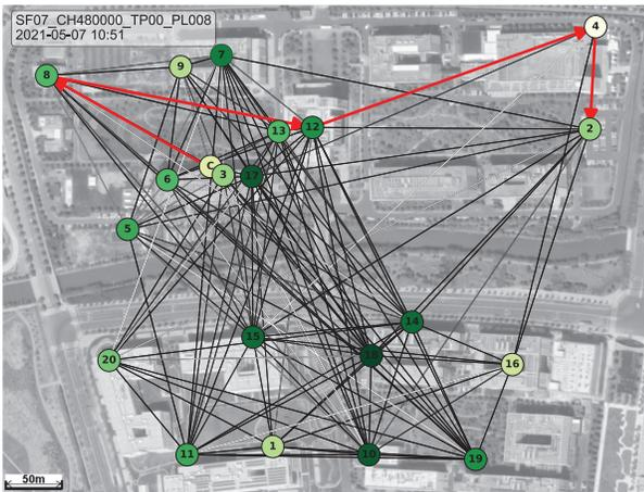
Figure 1: Location of the 21 nodes deployed using ChirpBox.
