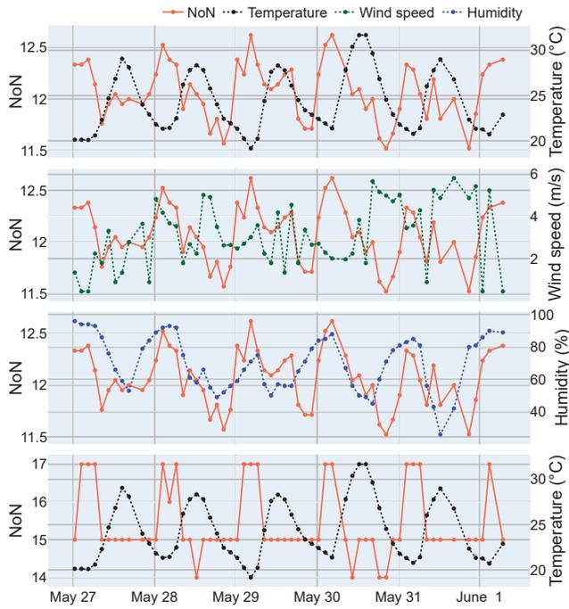
**Figure 4: Impact of various weather conditions on the average number of neighbours (NoN) in the network (top three plots) and on the NoN of node 13 (bottom plot) over 6 days. We employed RF channel 480 MHz and SF=7.**
