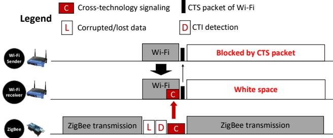
Fig. 2. In BiCord, ZigBee nodes sensing the presence of Wi-Fi traffic use cross-technology signaling to notify their need to access the channel. Nearby Wi-Fi devices understand the channel request and generate a white space.
