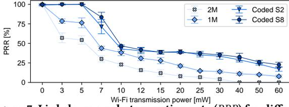
Figure 7: Link-layer packet reception rate ( $PRR$ ) for different PHY modes and interfering Wi-Fi transmission power. Note the non-linear  $x$ -axis scale showing the Wi-Fi transmission power.
