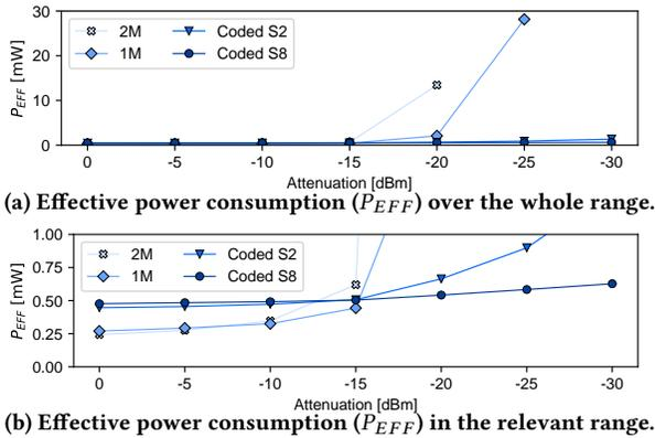
**Figure 9: Effective power consumption ( $P_{EFF}$ ) as a function of the used PHY and antenna attenuation of a BLE slave using a connection interval of 125 ms. Note that (a) shows  $P_{EFF}$  over its whole range, while (b) shows the range relevant for analysis.**
