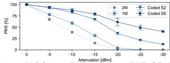
**Figure 6: Link-layer packet reception rate (PRR) of the BLE connection for different PHY modes and attenuation values.**
