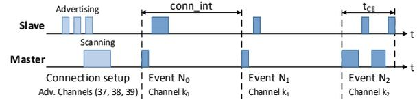
Figure 2: BLE connection between a slave and a master.
