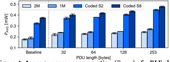
**Figure 4: Average power consumption ( $P_{AVG}$ ) of a BLE slave for different PDU lengths and PHY modes when using a fixed connection interval of 125 ms.**
