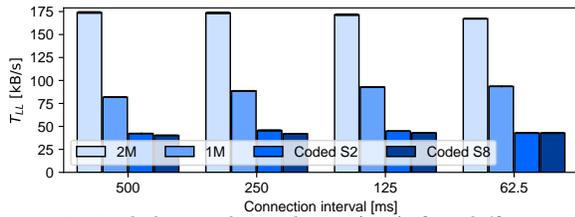
**Figure 5: Link-layer throughput ( $T_{LL}$ ) for different PHY modes and connection intervals measured at the master. Note that the standard deviation is at most  $\pm 0.4\%$  in our tests and, therefore, not clearly visible in the figure.**
