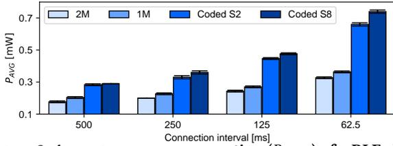
**Figure 3: Average power consumption ( $P_{AVG}$ ) of a BLE slave for different connection intervals and PHY modes when using a fixed PDU length of 253 bytes.**
