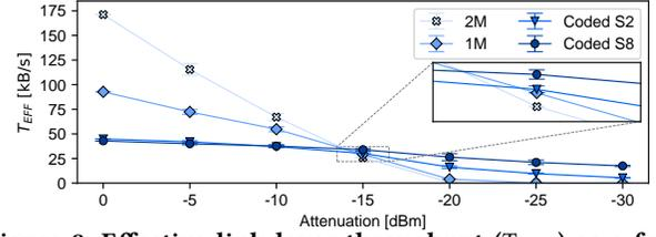
Figure 8: Effective link-layer throughput ( $T_{EFF}$ ) as a function of the PHY mode and the attenuation of the BLE slave antenna when using a connection interval of 125 ms.
